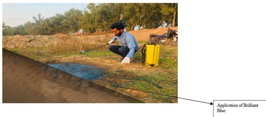
Fig. 2 Application of Brilliant Blue with hand pump
